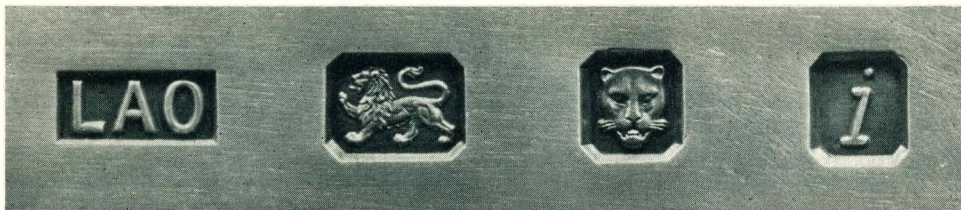
Silver marks: LAO, equivalent of maker's mark (here London Assay office); lion passant denotes sterling silver; leopard's head, town mark for London; and date letter for 1964-5.
