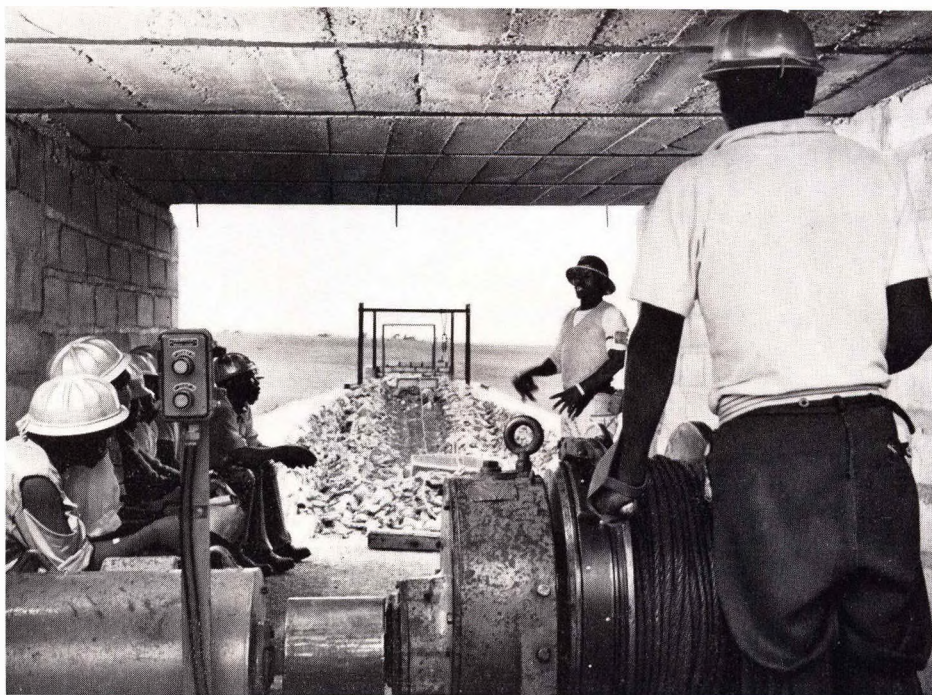
New African mineworkers being taught to operate a scraper winch at the Western Deep Levels training centre
