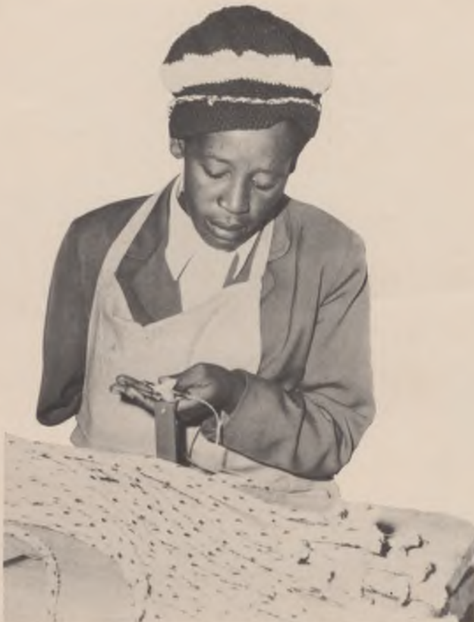
Whipping the ends of sisal lanyards for railway truck tarpaulins Die ente van sisaltoue vir spoortrokseile word beset.
