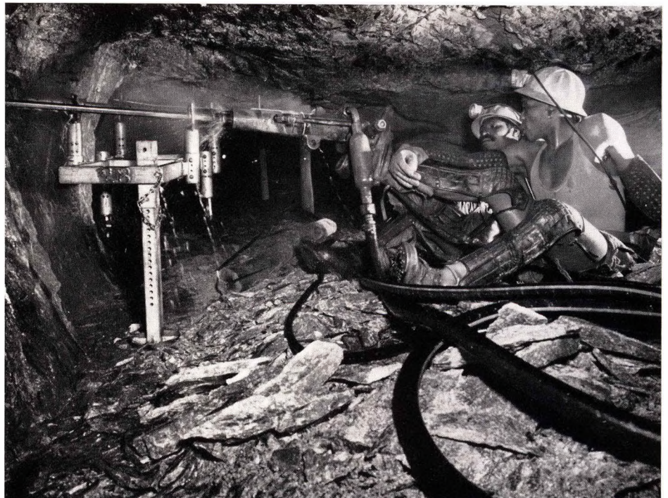
Drilling in a stope at Western Holdings, using steel stems tipped with tungsten carbide
