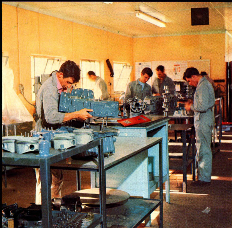
Modern aircraft engines are as reliable as any motor can be made. But they go through regular routine checks, with a complete strip for a major overhaul at around 2,000 hours, when parts, such as bearings, valves and seals, are automatically replaced irrespective of whether they are worn. The scene here is in the Placo engine workshop at Wonderboom.
