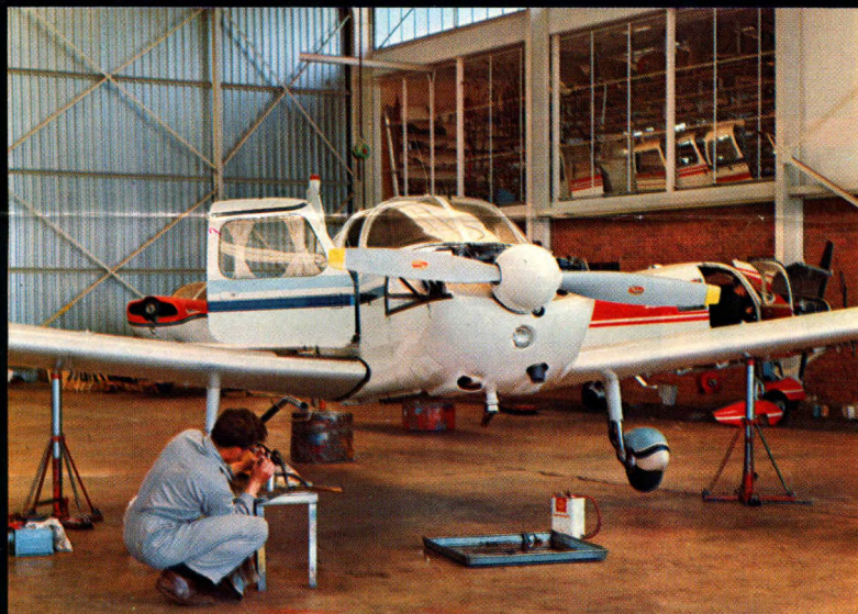
Constant mechanical checking is the order of the day with all aircraft at Placo. A Piper Cherokee 180 is up on jacks for checking the nose wheel.
