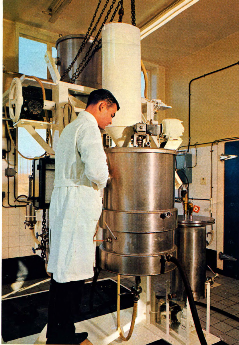
Mr. Bruno Brynard, the Pilot Brewery Supervisor, mashing in. The large stainless steel vessel in the foreground serves a threefold purpose serving as a mash tun, copper and hot wort receiver.
