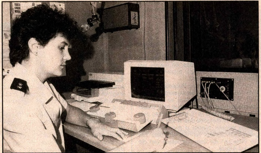
Lt S.C. Putter, of the Audiology Department, at the Maica Hearing Instrument used to test aspirant pilots' hearing. Regular testing provides records which can be used to track any deterioration in hearing over periods of time.
